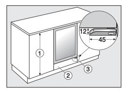
If adjacent furniture housing doors ① are taller than the wine conditioning unit door, the wine conditioning unit can be aligned to the unit doors using a filler panel ②.
